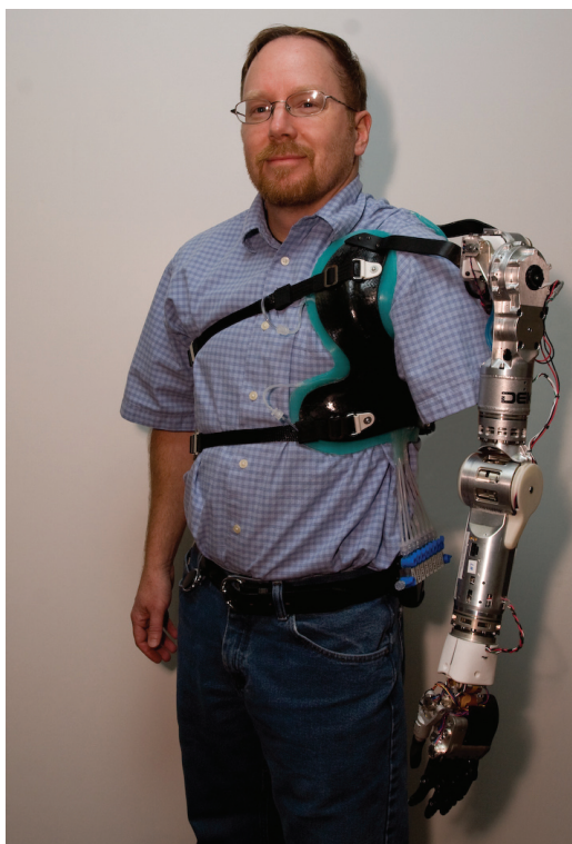
FIGURE 3.10 Conceptual model of DARPA's artificial arm that would be wired to the peripheral nervous system. SOURCE: DEKA Research and Development Corporation.
